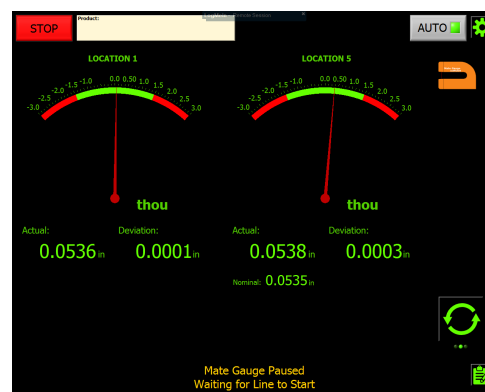
Needle Gauge Location Showing Left-Right thickness.
