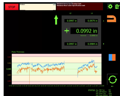
Display showing thickness at locations, and dual-location run chart.
