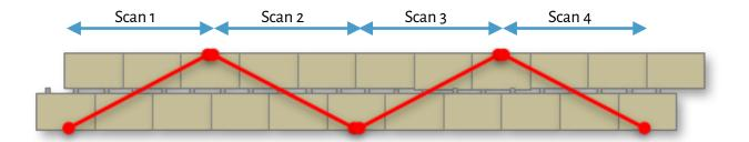
"Scan Capture" mode performs simultaneous strip traversal and continuous thickness measurements.
